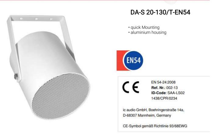
The 20W powered speaker is equipped with a 130mm full-range loudspeaker and a 100V line transformer with 4 power adjustments. A robust powder coated aluminum housing in RAL 9010, and a solid aluminium mounting bracket ensures the permanent installation of this speaker. For additional reliability, a 2 pinceramic block and a thermal fuse is provided in a junction box and the speaker chassis is impregnated against wetness.
