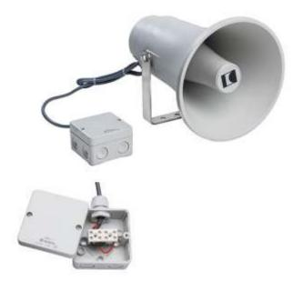
The 15W powered speaker is equipped with a 100V line transformer with 4 power adjustments, also lowimpedance operation (20ohm) is possible. The impact-resistant ABS housing UL94V0 in RAL 7035 guarantees long-term stability. For additional reliability, a ceramic block and a thermal fuse is provided in a junction box.
