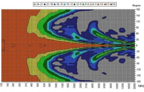
Parameters: Cyclic Move: 0°; Symmetry: average sym; Freq.Smooth: 1/3 Oct; Ang.Resol.: 5°; Rel. to: 0°Axis
